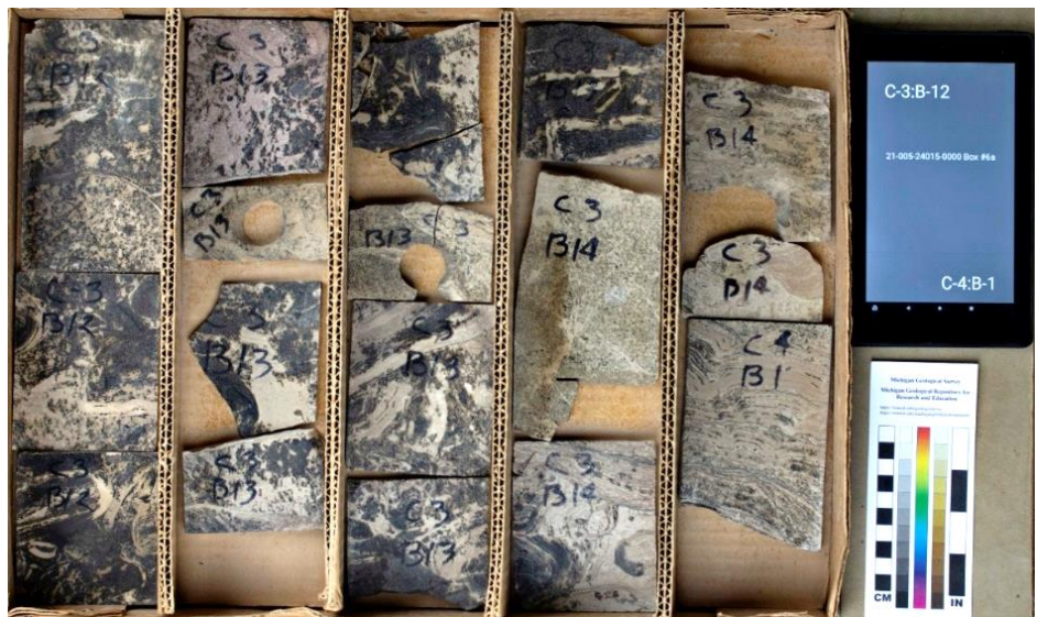
Fig. 2. Pinnacle reef facies with tarry residual oil staining from approximately 1,750-1,755' deep.
