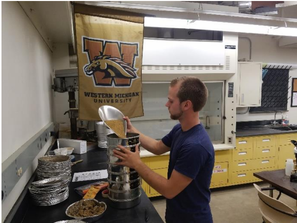
WMU student sieve testing samples in a lab
