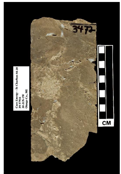
Figure 5: Bass Islands Dolomite in the layer with very high porosity and permeability
