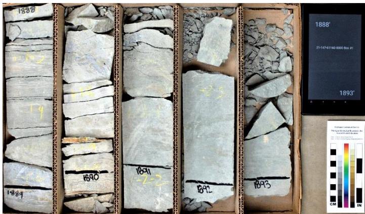
Figure 2: Middle C-Shale slabbed core from Consumers Power Brine Disposal #1-7 (depth in feet). From online collection of Michigan Cored well photos ( https://scholarworks.wmich.edu/core_photos/5836/ )
