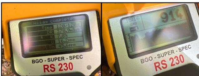
Figure 6. RS-230 BGO Super-SPEC Handheld Gamma-Ray Spectrometer. Top photographs of assay mode (left) and survey mode (right) taken by Nolan Gamet. Bottom photograph taken from Mount Sopris.com shows gamma spectrometer along with its rugged field case.
