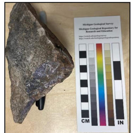
Figure 4. Fluorite-bearing, magnetic, quartz-feldspar-biotite schist collected by the mapping team this season. Fluorite-bearing samples are especially interesting because they may indicate the presence of rare Earth elements (REEs). Photograph by Nolan Gamet.
