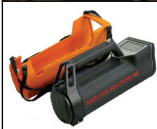
Figure 6. RS-230 BGO Super-SPEC Handheld Gamma-Ray Spectrometer. Top photographs of assay mode (left) and survey mode (right) taken by Nolan Gamet. Bottom photograph taken from Mount Sopris.com shows gamma spectrometer along with its rugged field case.
