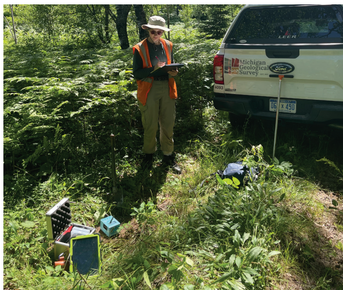
Emily Ratvasky, deploying a Tromino seismograph as part of a passive seismic survey for determining Quaternary sediment thickness in northern Dickinson County, Michigan.
