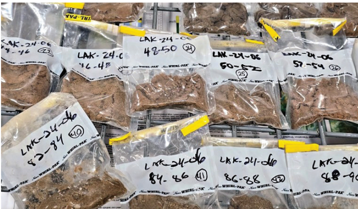
Sediment samples from Peacock quadrangle, collected in 2-foot increments down to 100 feet below the surface.
